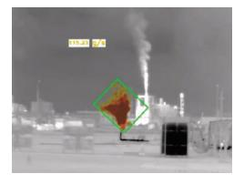
Leak flow rate 100 gr/sec (360 kg/h) of CH4 at 100m
