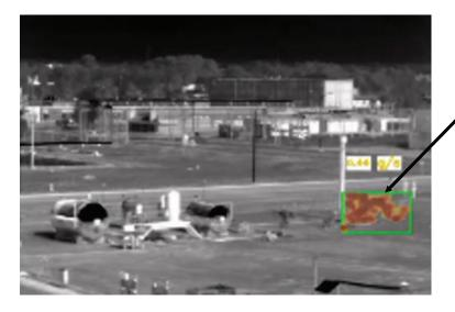
Leak flow rate : 0.45 gr/sec CH4 at 100 m
