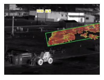
Leak flow rate 50 gr/sec (180 kg/h) of CH4 at 100m  $\,$
