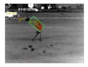
Leak flow rate: 0.32 gr/sec (1.15 kg/h) of CH4 at 50 m
