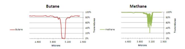
Our camera detects gases absorption of electromagnetic waves from any background Each gas has a specific absorption signature in the IR range.
