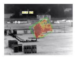
Leak flow rate: 200 gr/sec (720 kg/h) of CH4 at 100m
