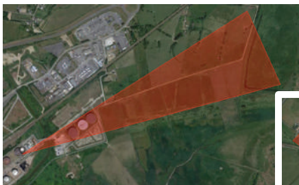
Multiple tanks roof monitoring using 1 or 2 cameras
