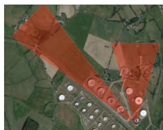
Multiple tanks roof monitoring using 1 or 2 cameras
