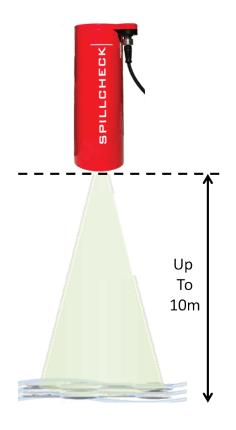
This technology allows us to detect oil film with minimum thickness from 1 to 10\*m (depending on the type of oil product) from a distance up to 10m (recommended distance being 3m).
