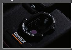
Infrared vision with a super sensitive 80x60 thermal sensor array, as standard
